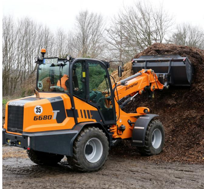
Unlike a classical wheel loader, the telescopic wheel loader has a much larger reach, piling up woodchips into high heaps, for example, to save storage space.
