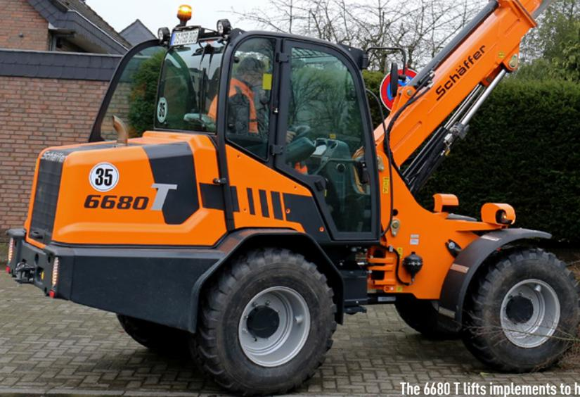
The 6680 T lifts implements to heights of 4.95m measured at the attachment pivot pin, which translates into an actual working height of six to seven metres or higher depending on the attachment.
