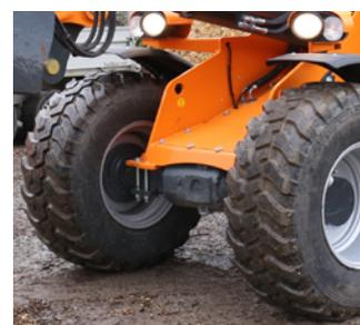
The MPT tread of the 20in tyres offers plenty of grip both on tarmac and on slippery ground.
