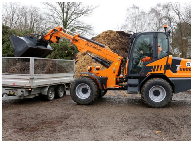
One of the typical tasks of the telescopic wheel loader – telescoping to a 4.95m height at attachment pivot pin, even larger trailers and trucks can be filled without difficulty.
