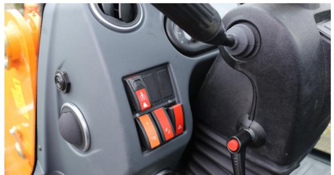
At a flick of the switch, the telescopic wheel loader is set to platform operating mode and this triggers a number of safety functions.
